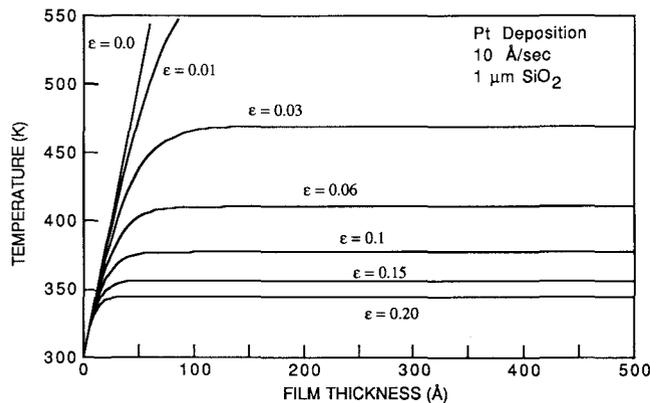
FIG. 2. Final cantilever-beam temperature as a function of deposited film thickness for various choices of total emittance.
