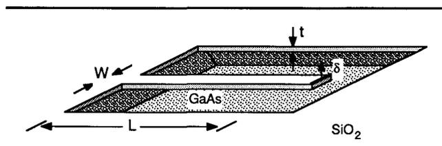
FIG. 1. Schematic diagram of a micro-cantilever beam.
