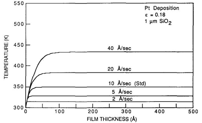
FIG. 3. Final cantilever-beam temperature as a function of film thickness for various deposition rates.
