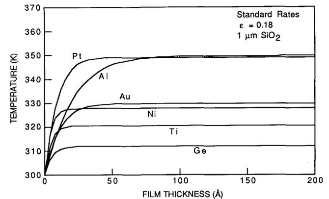
FIG. 4. Final cantilever-beam temperature as a function of film thickness for various elements deposited at the standard rates given in Table I.
