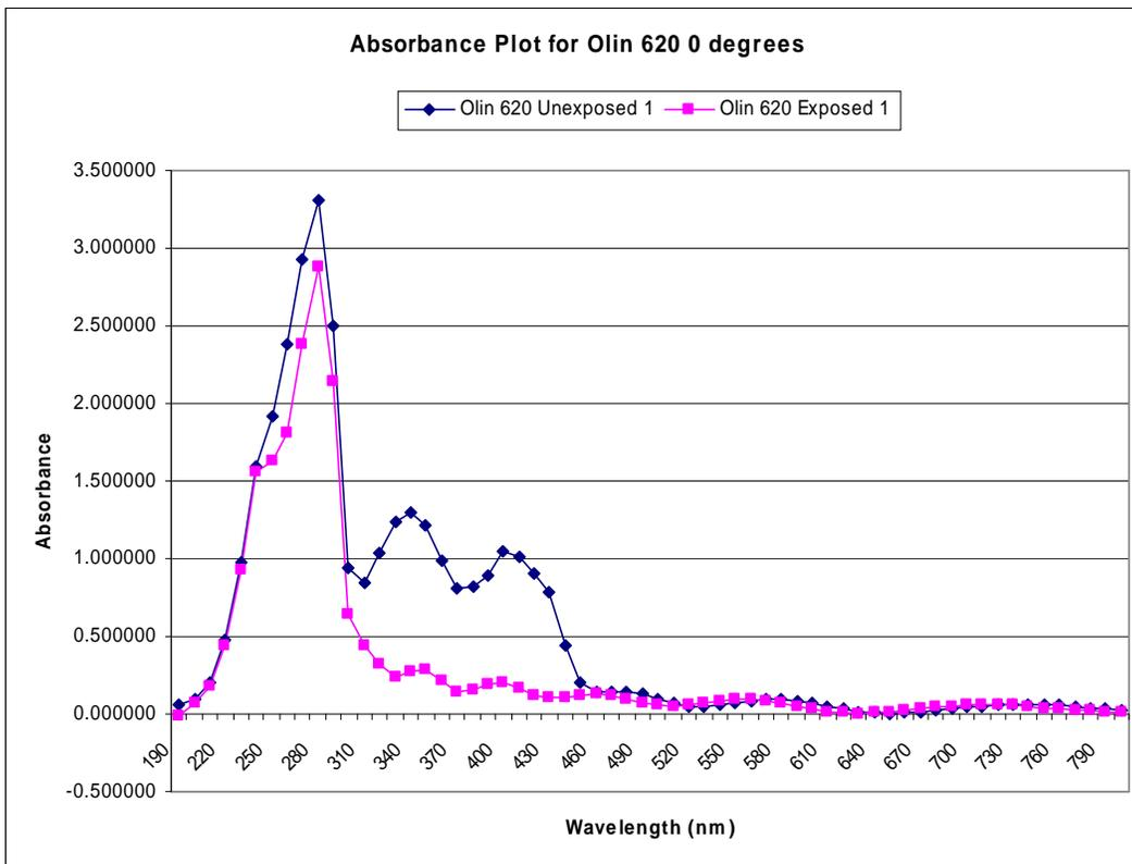
Figure 2: Plot of Absorbance vs. Wavelength for OiR620, rotated 0 degrees
