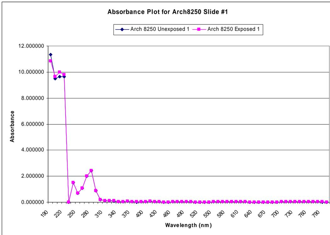
Figure 3: Plot of Absorbance vs. Wavelength for ARCH8250 DUV resist
