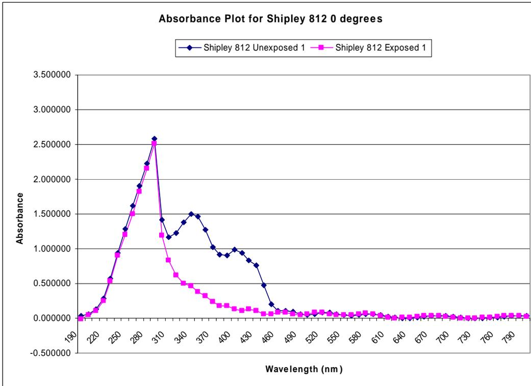
Figure 1: Plot of Absorbance vs. Wavelength for Shipley 812, Rotated 0 degrees
