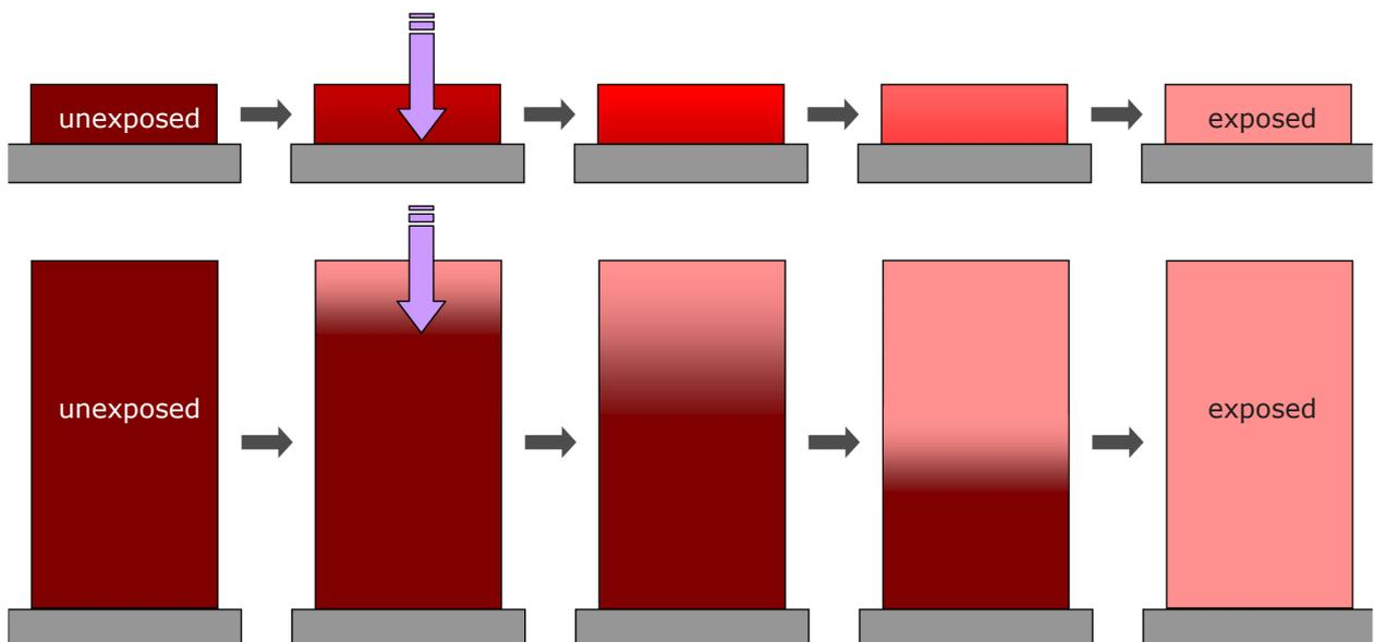
While "thin" resist films show a rather homogeneous illumination depth profile (top), 'thick' resist films bleach towards the substrate during exposure (bottom).
