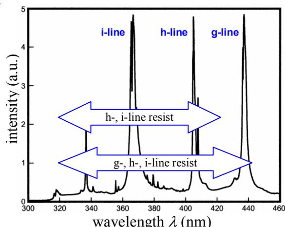
The absorption spectrum (spectral sensitivity see next section) of AZ® and TI photoresists is matched to this Hg emission spectrum.
