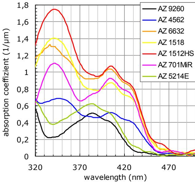
During exposure, positive photoresists almost completely bleach down to approx. 300 nm (fig. bottom):
