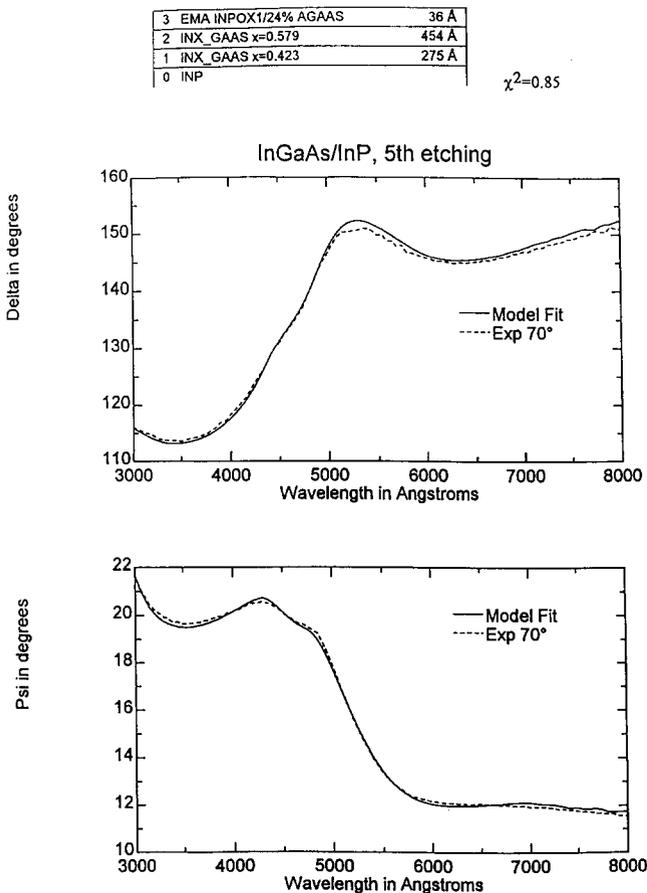
Fig. 3. Spectral  $\Psi$  and  $\Delta$  data for  $\text{In}_x\text{Ga}_{1-x}\text{As}/\text{InP}$  after etching in  $\text{CCl}_2\text{F}_2-\text{O}_2$ .
