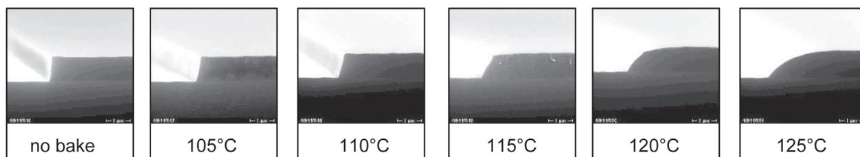
Cross-section of AZ<sup>®</sup> ECI 3000 resist structures suffering from an increasing temperature. *Source: AZ-EM<sup>®</sup> AZ<sup>®</sup> ECI 3000 Product Data Sheet*
