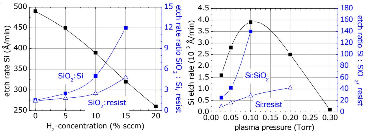
These plots show how dry etching parameters impact the Si and SiO<sub>2</sub> etch rate.
