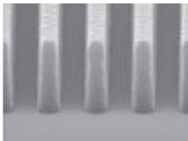
300 nm lines and spaces with the AZ® 701 MiR @ 0.8 µm
