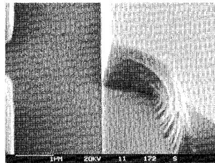
Fig. 11. SEM micrograph showing a part of a nitride line on top of a thin  $\text{SiO}_2$  layer. A part of the resist has been removed to demonstrate the anisotropy of pattern transfer.
