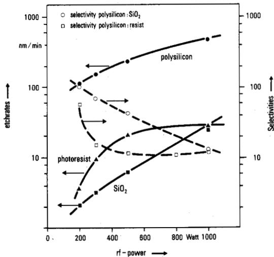
Fig. 2. Etch rates and selectivities on a logarithmic scale as a function of RF power. SF<sub>6</sub> is diluted with He at a ratio of 1:2. All etch rates are for a single 100-mm wafer.
