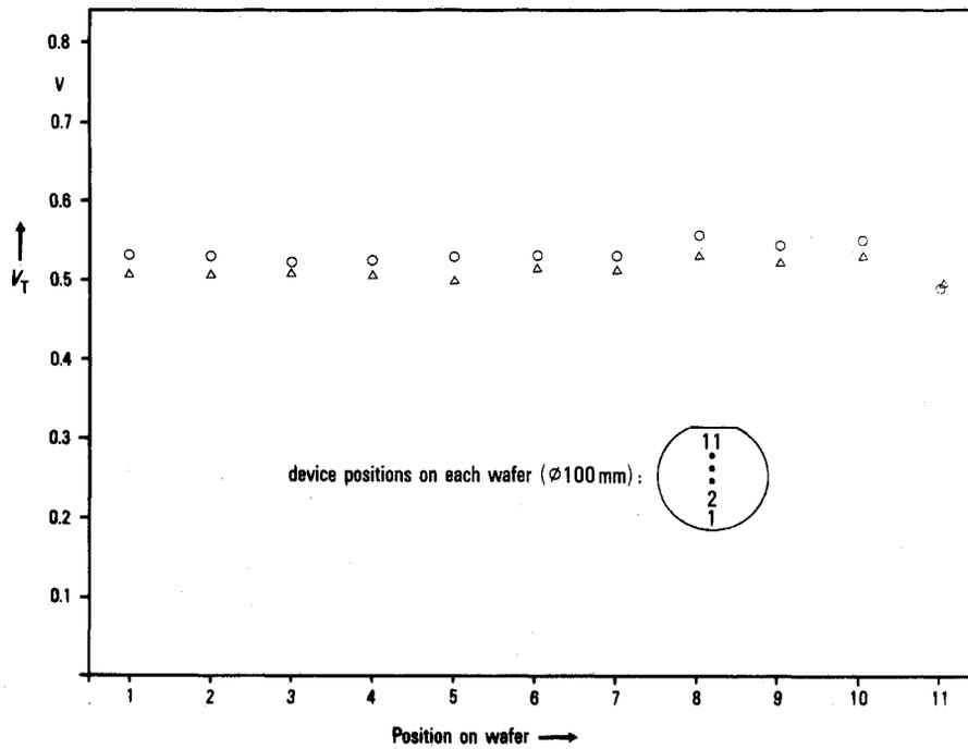
Fig. 7.  $V_T$  variation of a test MOS transistor ( $W/L = 30/3$ ) measured on 2 wafers ( $\Delta$ -no. 1,  $\circ$ -no. 27) randomly selected from a lot. The insert shows the measurement positions on the wafer.
