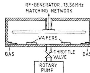
Fig. 1. Schematic diagram of the radial-flow batch-type reactor.
