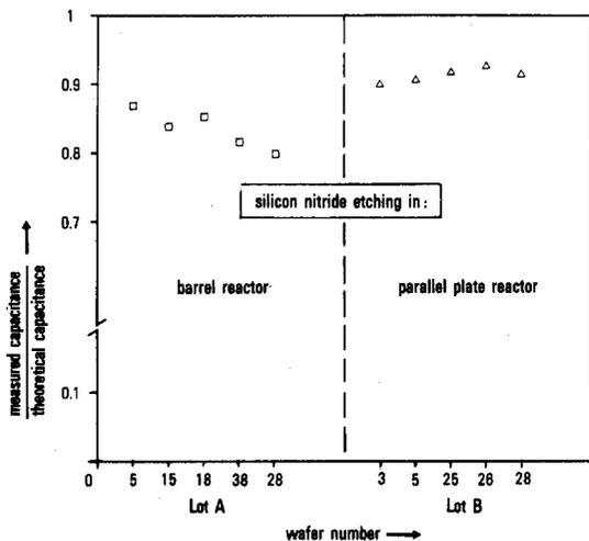
Fig. 12. Normalized storage capacitance of a memory-cell test array in standard MOS technology and its dependence on nitride etching process in different reactor types. Wafers have been taken at random from two different lots.
