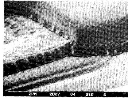
Fig. 5. SEM micrograph showing a part of a highly integrated MOS device where the polysilicon-2 layer has been strictly anisotropically etched (RIE) using  $\text{SF}_6$ . Note the ribbon at the polysilicon-1 edge.
