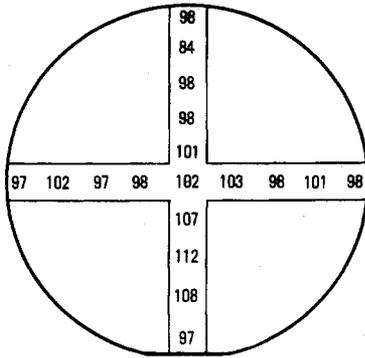
Fig. 9. Thickness of gate oxide (in angstroms) measured on 18 chips of a 3-in wafer after polysilicon etching. Oxide thickness has been determined prior to polysilicon deposition (110 Å in the center of the wafer).
