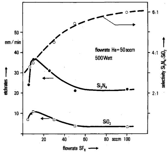
Fig. 10. Etch rates for  $\text{Si}_3\text{N}_4$  and thermal  $\text{SiO}_2$  and the corresponding selectivity as a function of  $\text{SF}_6$  gas flow.
