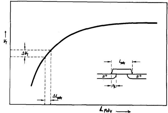
Fig. 6. Dependence of threshold voltage  $V_T$  on channel length  $L_{\text{Poly}}$  of MOSFET's (schematically). The quantitative "short-channel effect" is strongly influenced by specific fabrication steps.
