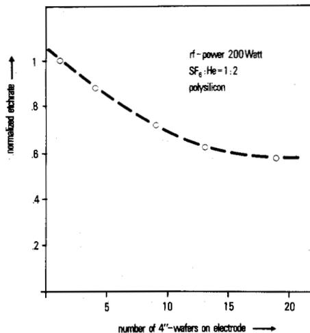
Fig. 3. Loading effect for polysilicon etching. Etch rates are normalized to the value for a single 100-mm wafer.
