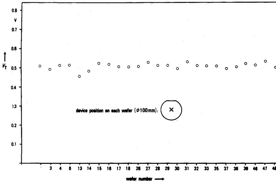
Fig. 8.  $V_T$  variation of the same test device as in Fig. 6 ( $W/L = 30/3$ ) over 25 wafers selected at random from one lot. The device position on the wafers is shown in the insert.
