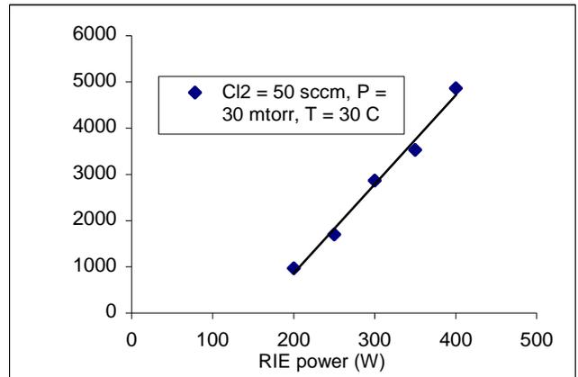
**Fig. 1** Etch rate of p-doped polysilicon against RIE power
