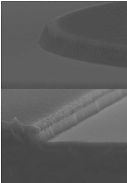
**Fig. 3** SEM photographs of RIE-etched p-doped polysilicon structures (2  $\mu\text{m}$  etch depth)
