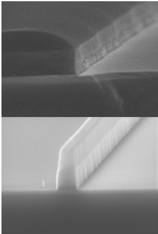
**Fig. 4** SEM photographs of RIE-etched p-doped polysilicon structures ( $2\ \mu\text{m}$  etch depth) using HBr.
