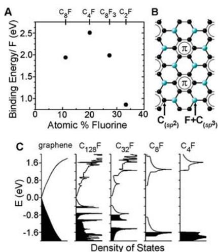
FIGURE 3. (A) Calculated binding energy per F atom compared to the  $\text{F}_2$  gas state. (B) Sketch of the calculated  $\text{C}_4\text{F}$  configuration for the 25% coverage from (A). (C) Calculated total density of states of single-side fluorinated graphene for several fluorine coverages.
