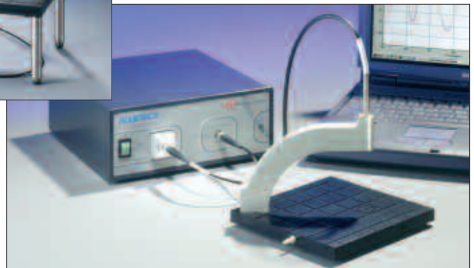
Transmittance maybe measured with a simple stage modification
