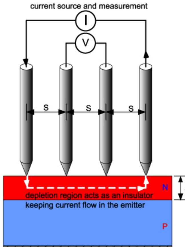
Use of a four point probe to measure the sheet resistivity of a solar cell.
